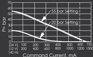
Pressure vs. Command (Range "D") 0.4 LPM Inlet flow
